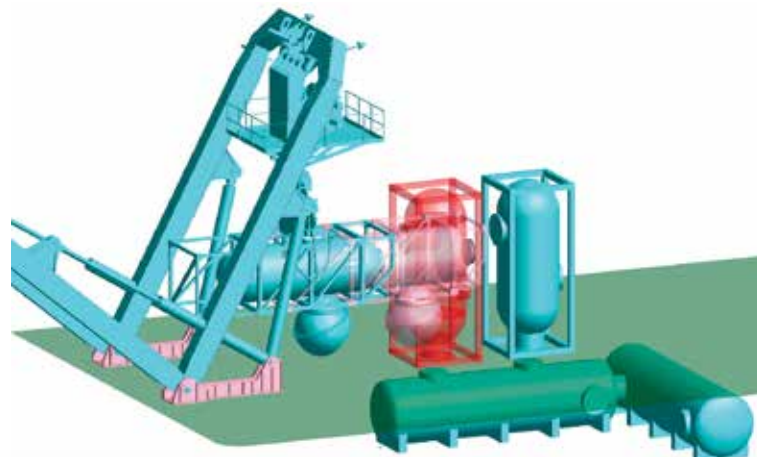
A-Frame, DTL and Chamber Arrangement
